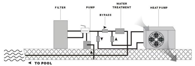
If your installation is equipped with a water treatment system such as a cell or injection port, the by-pass must be installed before the water treatment, with a non-return valve between the by-pass and water treatment system if required, refer Solarwise.
